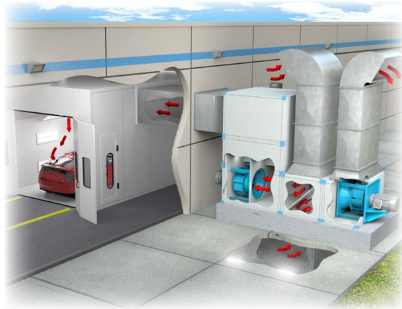
Paint Booth Ventilation
