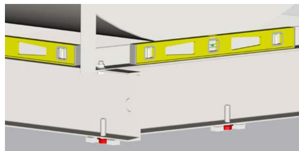
Carefully level the fan on the foundation
